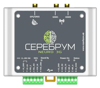
The GSM/GPS/GLONASS NEURO 3G module is an integrated communication module to provide YART and IRIS PLCs Internet telemetry connection. A complex GSM/GPS module inside gives online GPS/Glonass position and time information. These auxiliary positioning data become available in automatic mode whenever the Neuro module connection is established.
